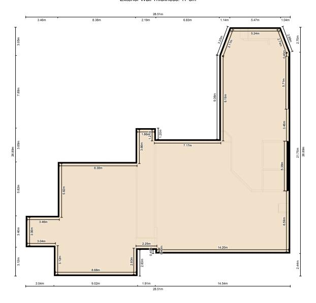
Measurement Diagram for: 1st Floor Exterior Wall Thickness: 17 cm
