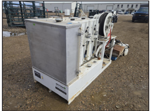
Western Enviro 5 Compartment Oil Dispensing Station (Unused)
