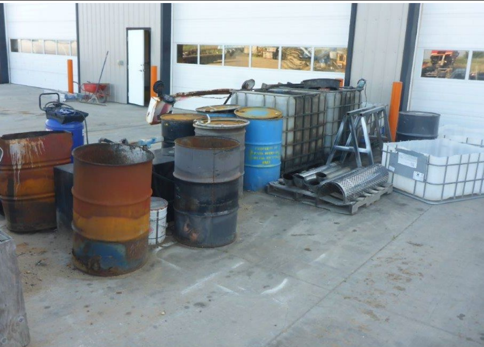
Photograph 16: The waste oil IBCs and drums used for the collection of oily rags, spent oil filters and emptied oil containers. One of the drums in the foreground contained ash from burned paper wastes.
